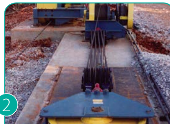
2 Main Barge Puller Style 1000 & Take-Up System
