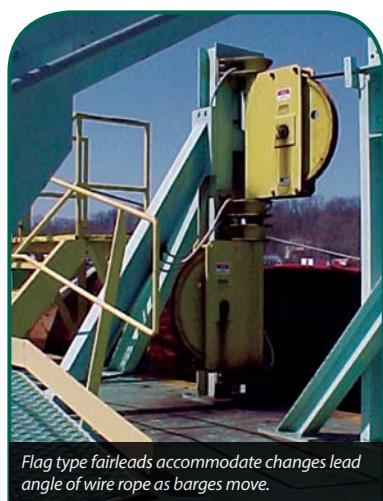
Four roller fairleads used to guide wire ropes to barges from breasting winches.
