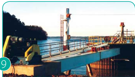
9 Barge Breasting Winch System
