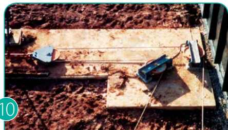
10 Railcar Puller Take-Up System
