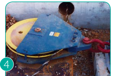
4 Barge Haul Horizontal Bend Sheave
