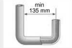
● Minimum clearance of U-shape bends
