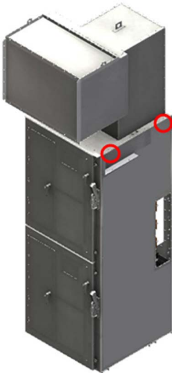
Figure 8: Install the upper bracket and secure it to the MCC
