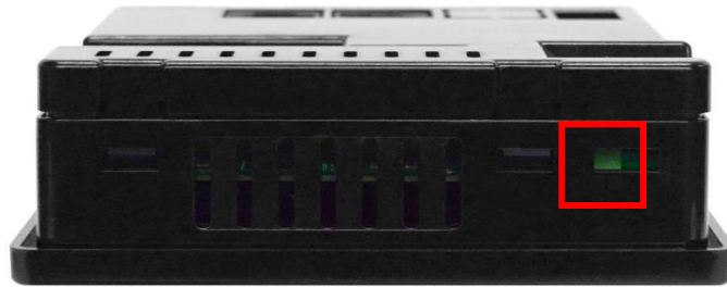
Figure 3.1 - X7 OCS with Mounting Clip Location
