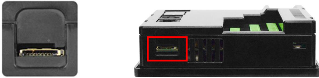
Figure 10.1 - Removable microSD Memory Card Slot
