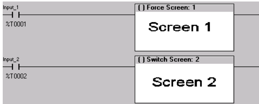
Figure 13.5- Force and Switch Coils in Ladder Programming
