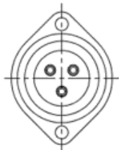
Amphenol PWF-03PMMS SC7001 connection in pump
