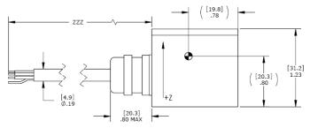
WIRE DESIGNATIONS: WHITE = INPUT (EXCITATION) BROWN = OUTPUT X AXIS GREEN = OUTPUT Y AXIS PINK = OUTPUT Z AXIS YELLOW = COMMON (CIRCUIT GROUND) GRAY = NO CONNECTION
