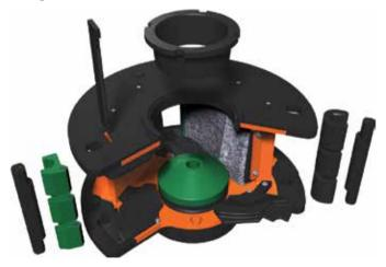
Components have been integrated when possible and the number of fixing points have been reduced to make the Orange Series Rotors easier to maintain.
