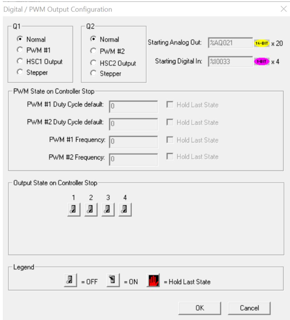
Figure 7.10 - Digital / PWM Output Configuration Dialog
