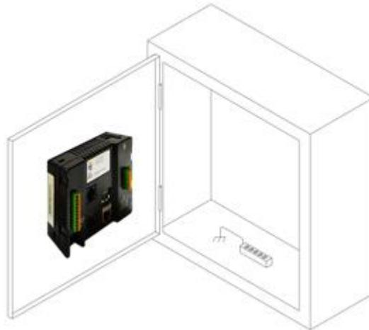
Figure 3.1 - Panel Mounting of an X5 Series OCS
