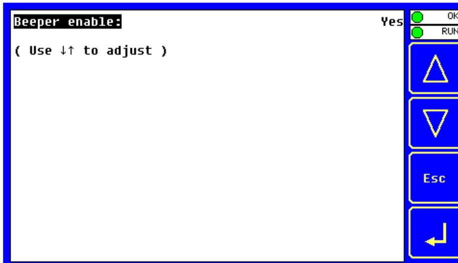
The Set Beeper Sub-Menu displays one System Setting, which is editable
