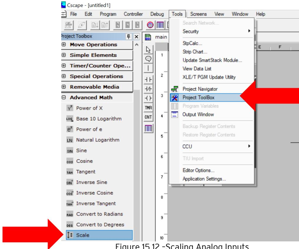
Figure 15.12 -Scaling Analog Inputs
