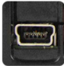
Figure 7.2- USB Programming Connector
