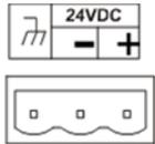
**Solid/Standard Wire:** 12-24 awg (2.5-0.2mm).
