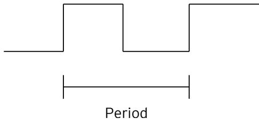
Figure 9.6--PWM, Two Parameters: Duty Cycle & Frequency
