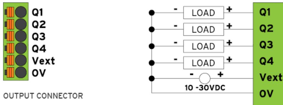
Figure 8.1- Typical Output Wiring
