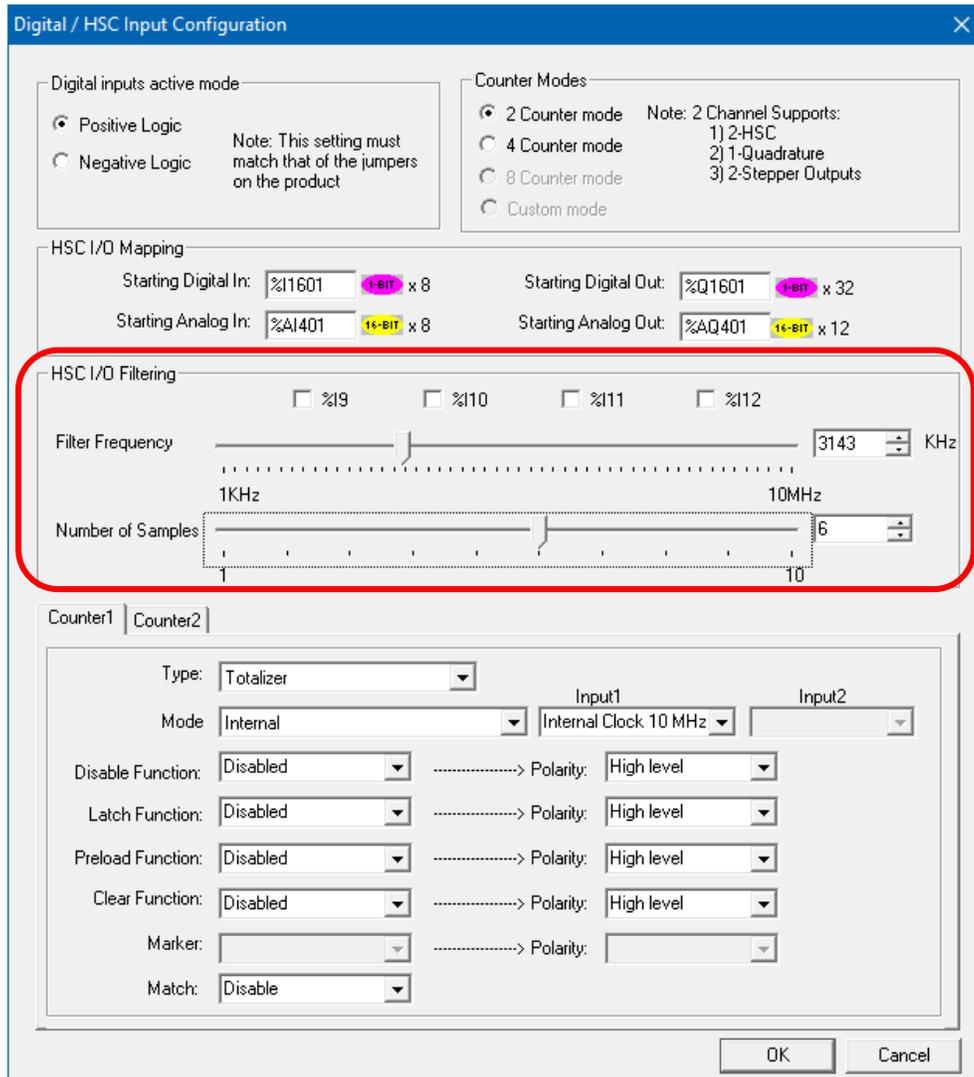
Input signal is filtered based on the filter frequency and Number of samples selected. User must select Filter Frequency and Number of samples based on the frequency of the Input signal.
