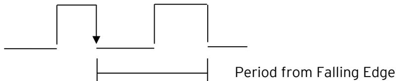
Figure 9.3 & 9.4--Period Measurement, Rising Edges & Falling Edges
