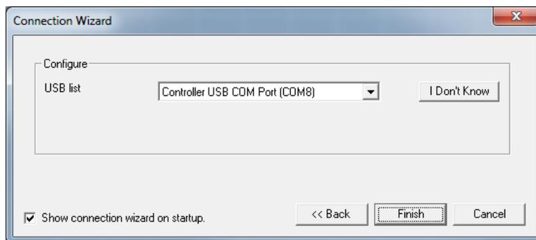
If the Connection Wizard does not pop up upon opening Cscope, then select **Controller** (in the Cscope tool bar) → **Connection Wizard**, choose your connection method. If you are connecting for the first time, we suggest connecting via USB.
