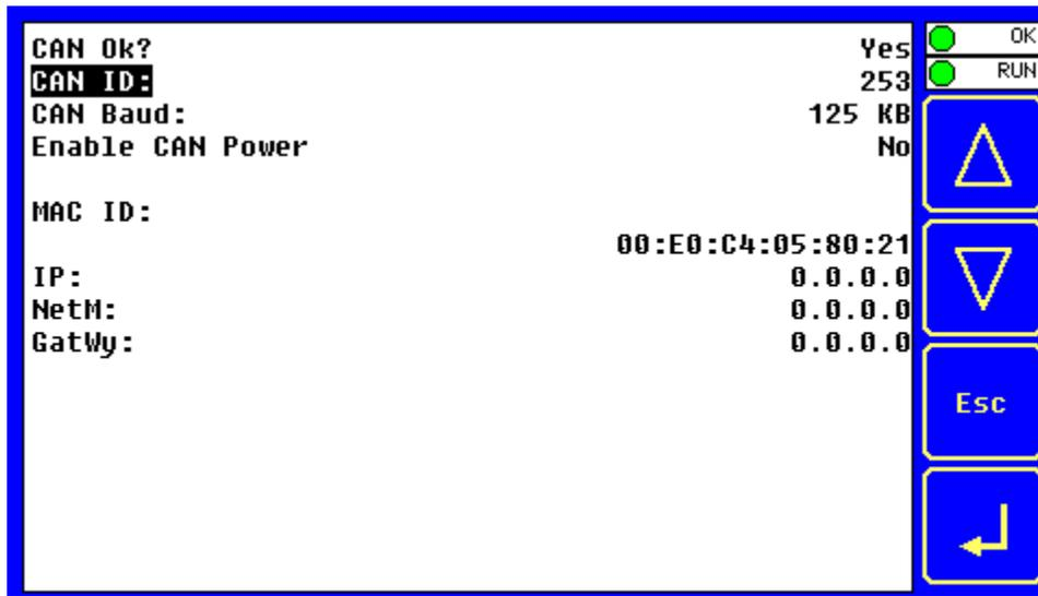
This sub menu allows setting for the CAN and Ethernet network to be viewed or changed.
