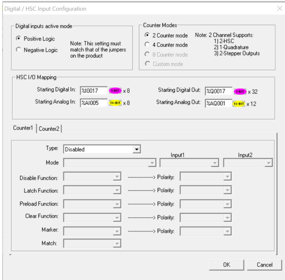
Figure 7.9 - Digital /HSC Input Configuration Dialog
