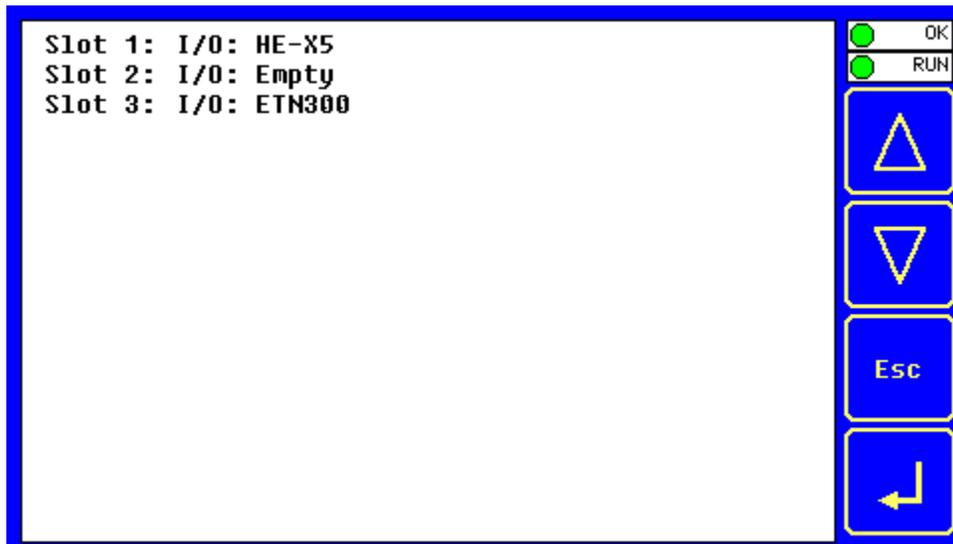
The View I/O Slots Sub-Menu displays three System Settings, all of which are not editable.
