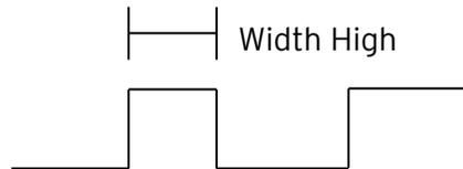
**Width Low 1  $\mu$ s Counts** - In this sub-mode the accumulator value will contain the number of 1  $\mu$ s counts the pulse is low.
