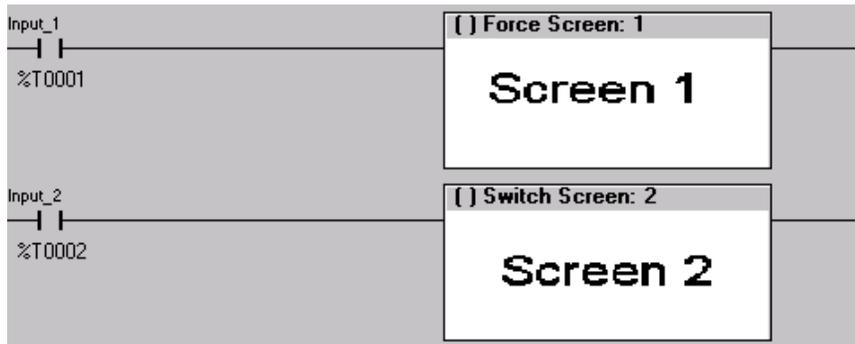
Figure 14.5- Force and Switch Coils in Ladder Programming
