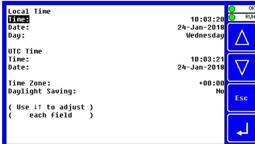
**To Set Time Zone:** The Time Zone setting is an hourly offset from UTC time. If using the Time Zone setting, set it first, then set the local time. UTC time will be automatically set based on the time zone and local time settings.
