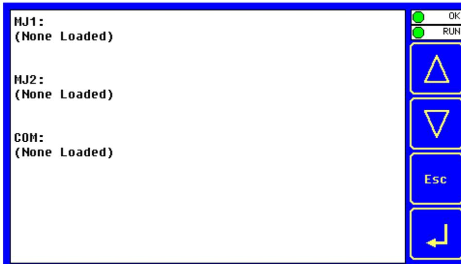
The View Protocols Sub-Menu displays protocols used on the ports, none of which are editable here.
