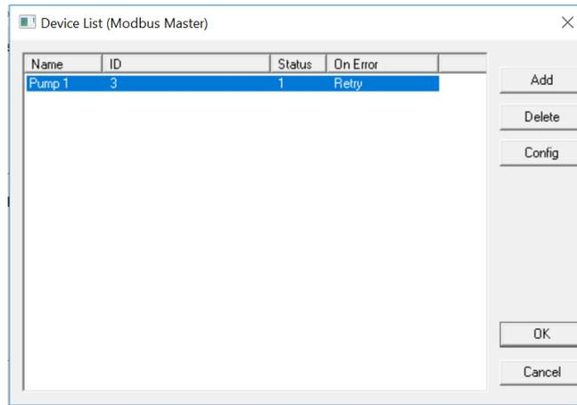
The Device List is reached from the Device button on the Protocol Config screen and provides a list of the configured devices on the Network. Devices must be created and exist in this list before corresponding Scan List entries can be created for this device. Typically, the number of entries is limited to **64 devices**.
