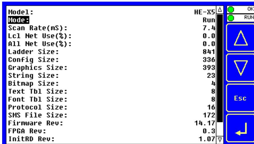
The View Status Sub-Menu displays up to 19 System Settings. Only the **Mode** System Setting is editable.
