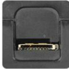
Figure 16.1- Removable microSD Memory Card Slot
