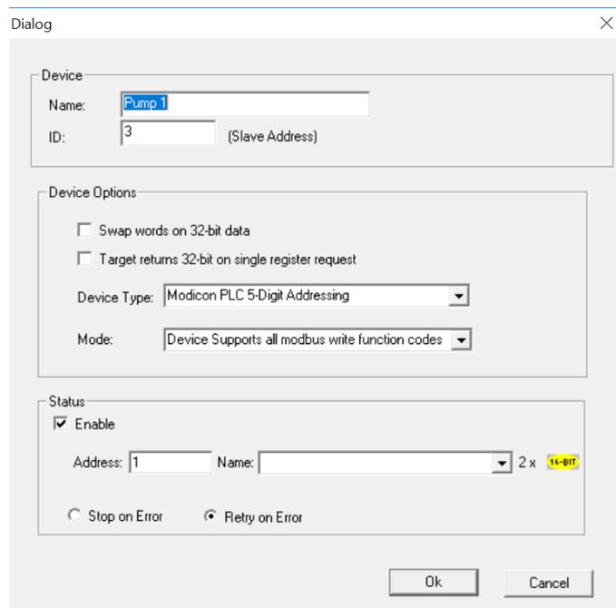
This configuration is reached from the Device List when adding or modifying an existing device.
