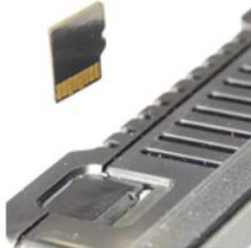
Figure 16.2 - Installing Removable Memory Card
