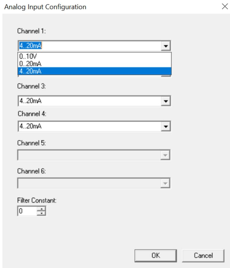
Figure 7.11 - Analog Input Configuration Dialog
