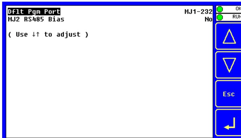
The Set Serial Ports Sub-Menu displays two System Settings, all of which are editable, and one optional item. For the **Dflt Pgm Port** System setting, only MJ1-232 can be selected.
