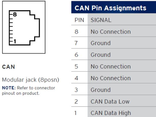
Figure 11.2 - CAN Port Connector
