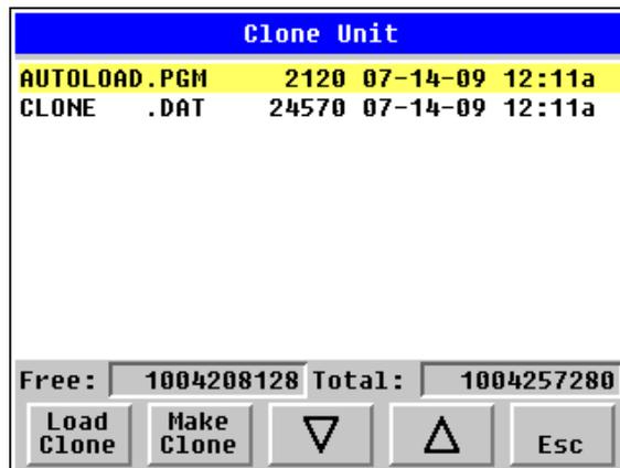
**NOTE:** For security enabled files, Load Clone asks for password validation before loading the application.
