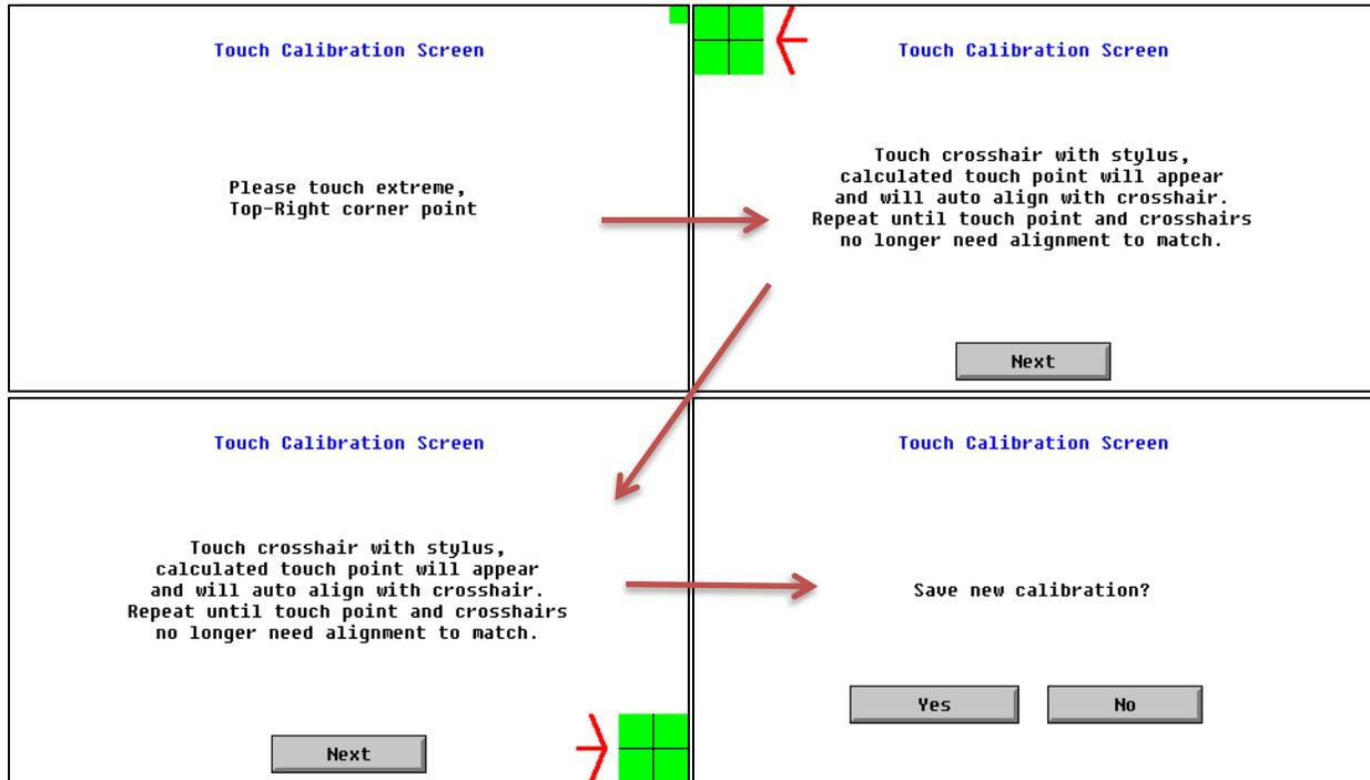
Figure 5.4–Screen Calibration
