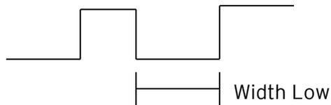
Figure 9.1 & 9.2- Pulse Width Measurements, High & Low
