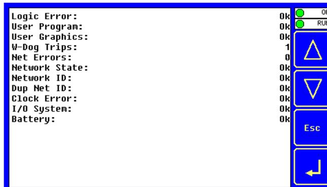
The View Diags Sub-Menu displays up to 11 System Diagnostics, none of which are editable.
