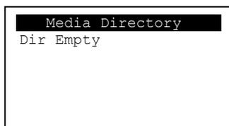
= microSD card is installed and initialized, but contains no files
