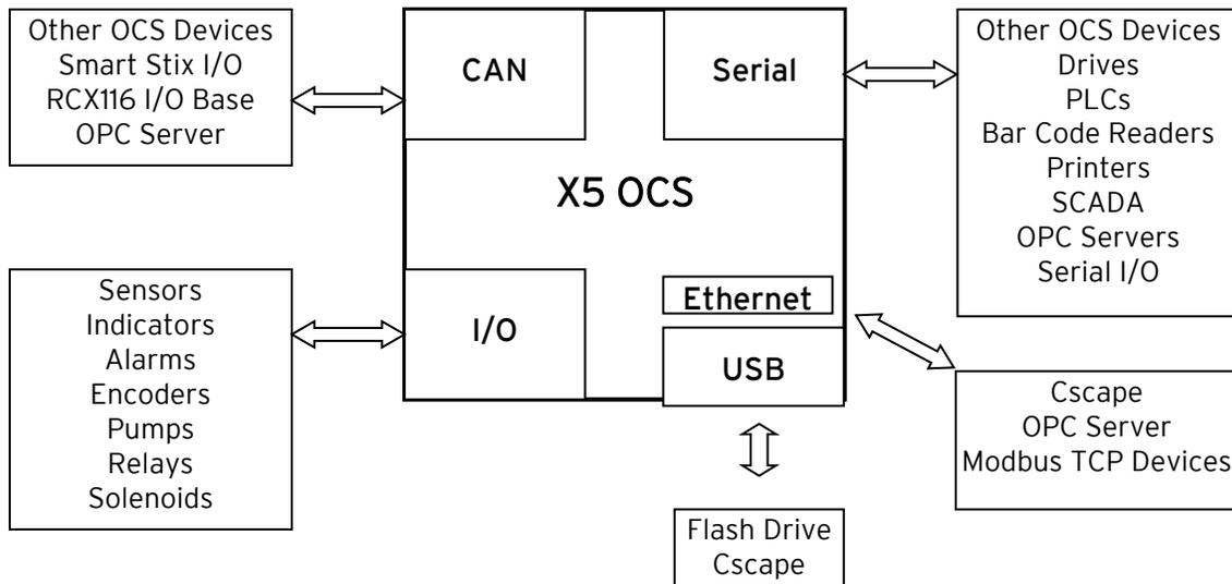
Figure 2.1 - Visual Overview of Types of Devices that can be connected to X5 OCS
