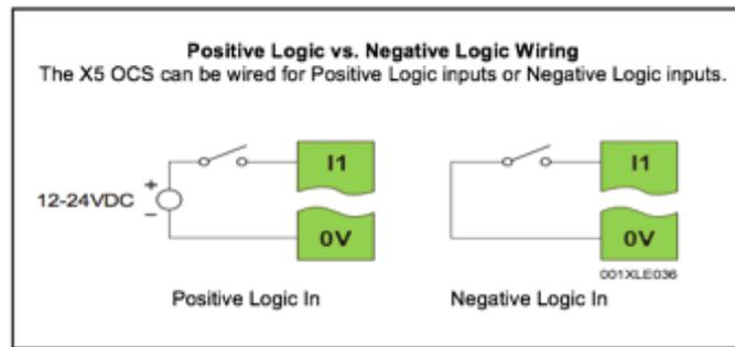
Figure 8.2- Positive and Negative Inputs
