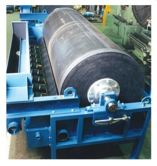
which decreases rapidly with the distance away from the drum. Hence, the smaller pole pitch (referred to as high gradient, HG) has a greater ability to pick up finer or less magnetic particles but has a lower throughput capacity when compared to a magnetic assembly with a larger pole pitch.
