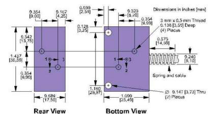
Two through holes and four 3 mm x 0.5 mm
