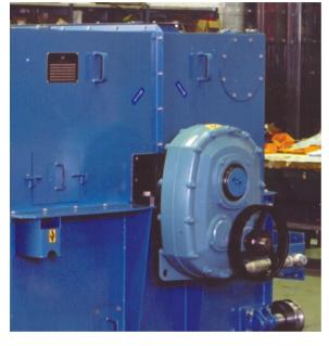
tom for discharge of both magnetic and nonmagnetic products. These products are separated by means of a splitter placed under the drum inside of the housing. The whole unit can be dust vented by connecting the plant exhaust system to the outlet provided on the housing.
