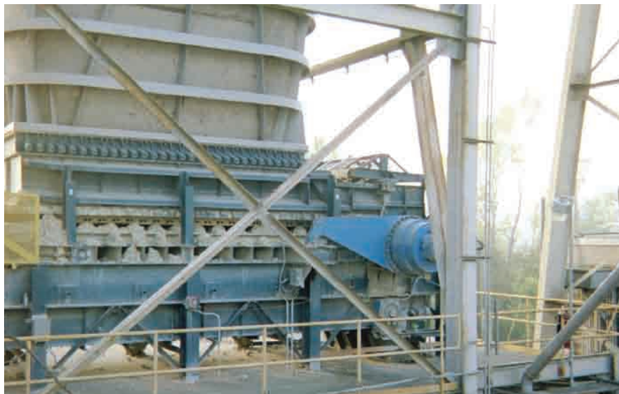
Apron Feeder at a major cement producer extracting clay from a storage bin.
