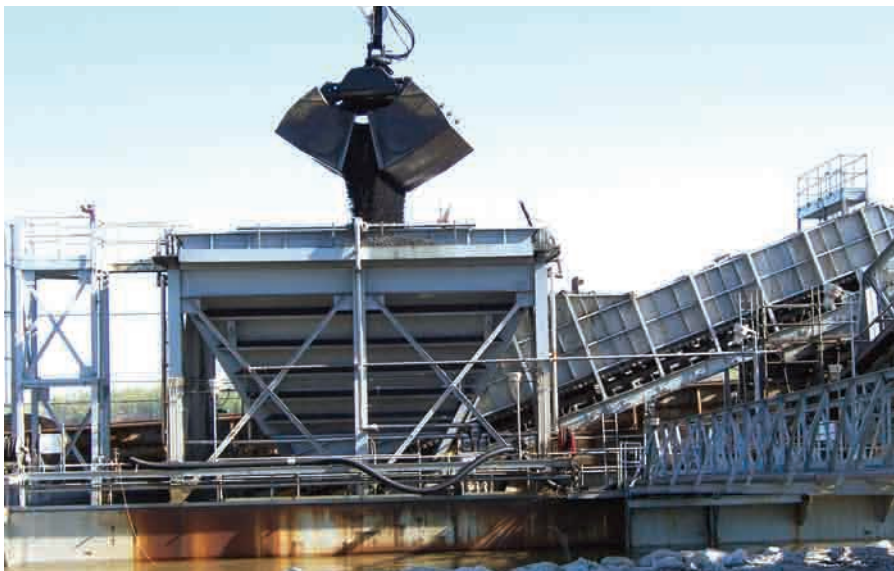
Apron Feeder extracting coal from a hopper on a floating barge to feed a major power plant.
