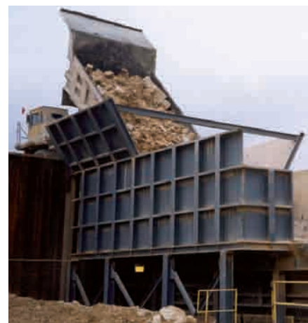
Truck dump hoppers utilize the Metso Apron Feeders to withdraw rock and ore at a controlled rate of speed to feed other equipment such as all types of crushers, vibrating grizzlies, wobbler feeders or conveyors.
