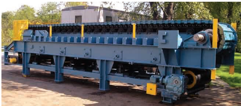
Metso manufactures Apron Feeders of various size, tonnage and drive configurations to meet the specific application and customer requirements.
