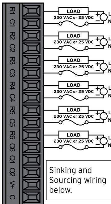
NOTE: Internal 10kΩ resistors between: V+ and Q1; V+ and Q2
