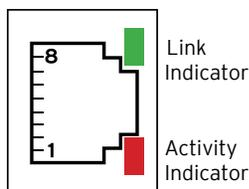
10/100 Ethernet port with automatic MDI-X (crossover detection) is provided via the single 8-position modular jack labeled "LAN". Several features are available for use over Ethernet: ICMP (Ping), EGD (Ethernet Global Data, Modbus Slave, Ethernet / IP, FTP (File Server), and ASCII over TCP/ IP.
