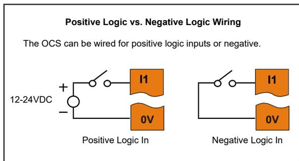
Digital inputs may be wired in either a Positive Logic or Negative Logic fashion as shown. The setting in the Cscape Hardware Configuration for the Digital Inputs must match the wiring used in order for the correct input states to be registered.
