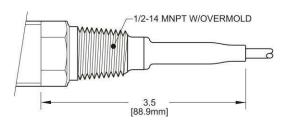
Strain relief with 1/2" Conduit Fitting
